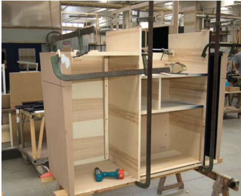
Banco cassa in costruzione / Cash counter under construction
